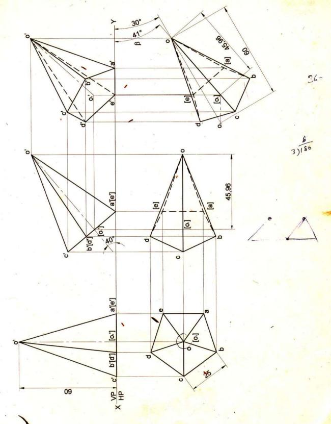
**Problem 22** A pentagonal pyramid 25 mm sides of base and 50 mm axis length rests on HP on one of its corners of the base such that the two base edges containing the corner on which it rests make equal inclinations with HP. Draw the projections of the pyramid when the axis of the pyramid is inclined to HP at 40° and appears to be inclined to VP at  $45^{\circ}$ .
