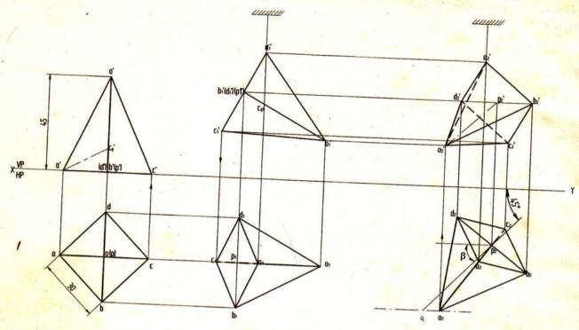
Problem 50 A cone of base dia. 40 mm and axis length 50 mm is resting on HP on a point on the circumference of its base such that its apex is at 40 mm above the HP and its top view of the axis is inclined at 60° to VP. Draw the top and front views of the solid. Also, determine the inclinations of the axis when the base Solution
